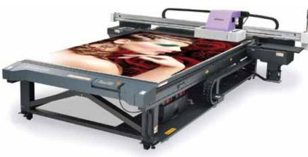
printers to print on flat substrates to eliminate the cost and labor to mount prints on vinyl. Very good for site signs, real estate signs, and virtually any type of flat sign or graphic,
