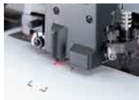
Light pointer easily adjust the head position to crop marks
