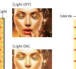
Single-layer printing looks faded when the illumination is on because too much light is transmitted.
