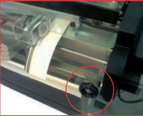
The new Y manual correction tool compensates roll winding and printing errors.
